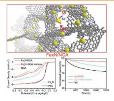
A novel macroporous iron nitride/nitrogen doped-graphene aerogel hybrid is reported as a highly active, stable, and low-cost catalyst for oxygen reduction reaction. The strong interactions between Fe<sub>x</sub>N nanoparticles and graphene substrates boost its performance. It is also found that surface area, porosity, density of Fe-N-C sties, and particle sizes affect electrocatalytic activity.
