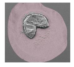
Robust microcapsules of carbon black suspensions high in solids loading (up to 0.2 g/mL) are prepared for electrical conductivity restoration. Octadecyl chains are covalently attached to carbon black surfaces to improve dispersability and suspension stability in o-dichlorobenzene. The microcapsules exhibit significant particle release upon crushing, resulting in full conductivity restoration of damaged silicon anodes.
