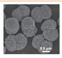
3D hierarchical ZnCo<sub>2</sub>O<sub>4</sub> twin spheres are prepared via a convenient polyol process and subsequent thermal annealing. A multistep splitting in situ dissolution recrystallization originating from 1D nanorods is first proposed to understand the formation of the 3D nanoarchitectures. Lithium-ion batteries prepared with the 3D materials display remarkable performance in energy storage.
