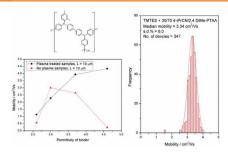
High mobility organic semiconductor formulations with excellent uniformity are prepared by combining a small molecule and high permittivity semiconducting oligomers. The use of these high-k (k > 3.3) oligomers allows control of the performance by manipulation of the surface energy of the substrate. Organic thin film transistors results with mobilities of 5 cm $^2$  V $^{-1}$  s $^{-1}$ , standard deviation <10% and on/off ratios of 109 are presented.
