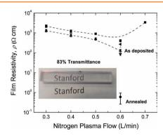
The successful deposition of conductive transparent TiN<sub>x</sub>/TiO<sub>2</sub> hybrid films on polycarbonate substrates is demonstrated in air using atmospheric plasma processing. The visible transmittance ranges from 71% to 83% and the film resistivity is in the range  $\sim 6.0 \times 10^{-1}$  to  $2.4 \times 10^5$  ohm cm. It provides a new promising way to fabricate transparent conductive films with low cost.
