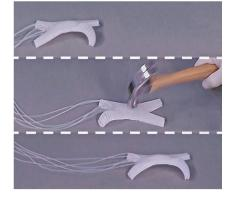
Soft pneumatic actuators and robots based on composites consisting of elastomers and embedded flexible reinforcing sheets are significantly more resistant to blunt impacts, tensile forces, and severe bending than hard robotic systems of similar size and weight. The range of physical damage that soft robots and actuators can withstand without suffering changes in mechanical performance is quantified.
