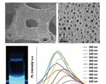
A facile and high-yield synthesis method for high quality and strongly photoluminescent graphene quantum dots (GQDs) by electrochemically exfoliating free standing three dimensional graphene foam is demonstrated. The synthesized GQDs are utilized for specific optical detection of ferric ions.
