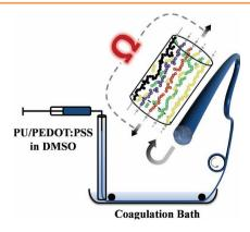
Conducting elastomeric fibers based on a composite of polyurethane (PU) and **PEDOT:PSS**, produced by a wet-spinning method, have high electrical conductivity and stretchability. These fibers can sense large strains by changes in resistance. The PU/PEDOT:PSS fiber is optimized to achieve the best strain sensing. PU/ PEDOT:PSS fibers can be produced on a large scale and integrated into conventional textiles by weaving or knitting.
